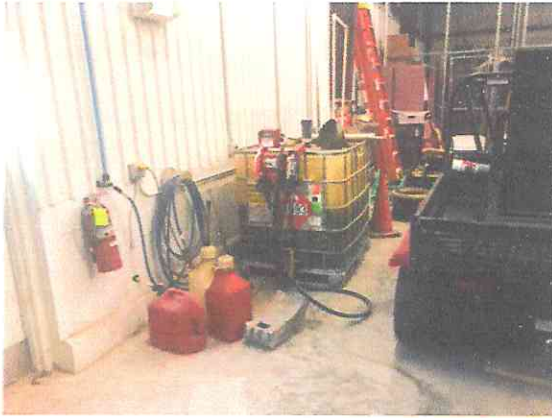
Photo #1: Cold Storage Building, south side of property. Bulk tank of Fuel treatment, as well as small fuel containers located out or traffic way.
