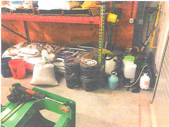
Photo #9: Spray canisters and buckets stored out of traffic way. Recommended secondary containment for sprayers not in use.
