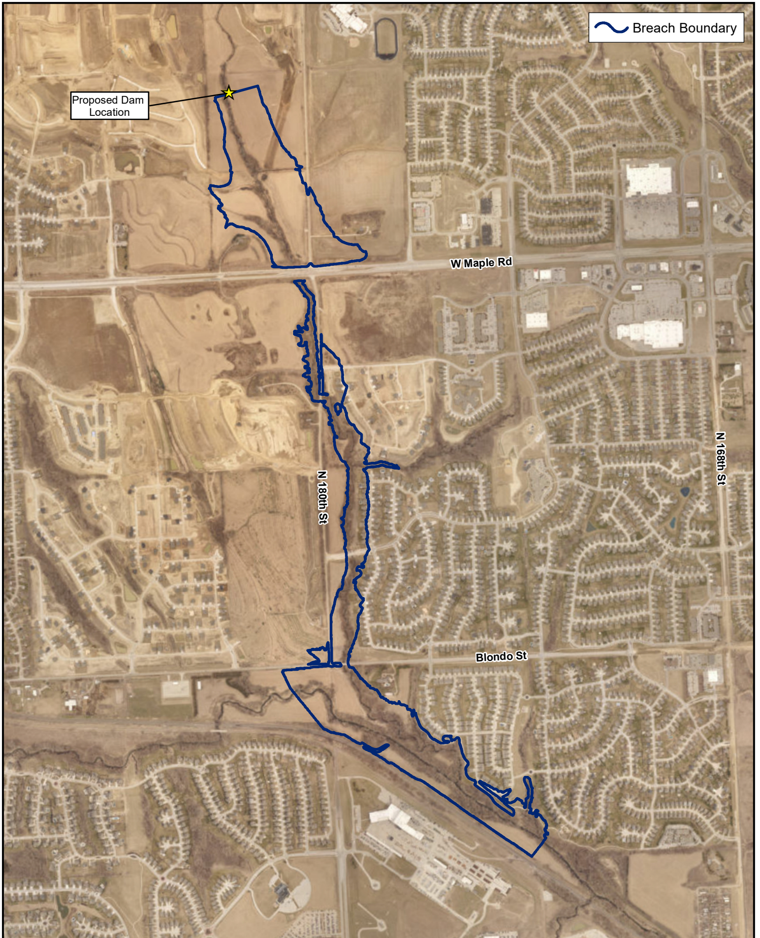
Figure C6.2. Site WP-1 - Breach Boundary
