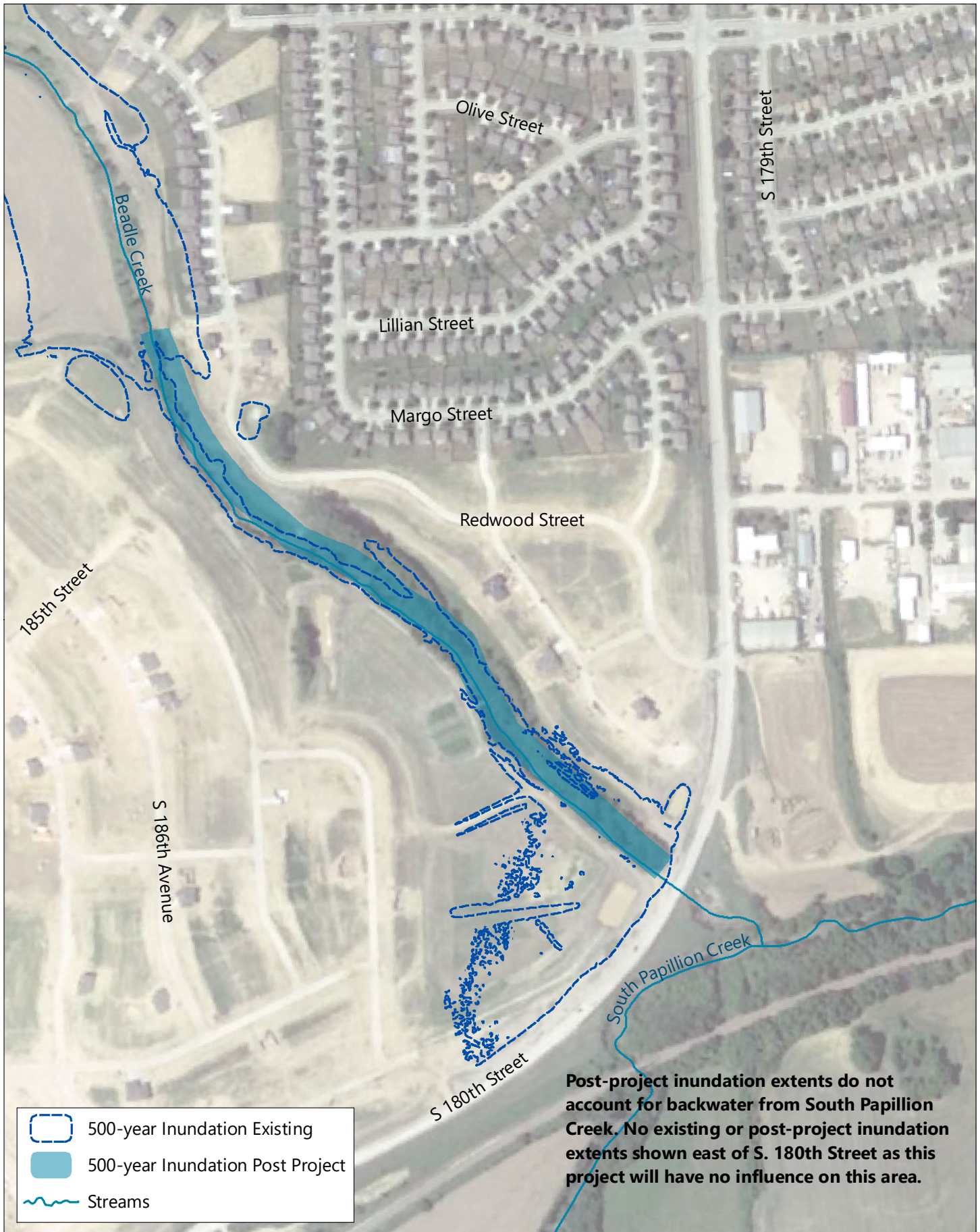
Figure C2.4. S-5 500-Year Flood Papillion Creek Supplemental Watershed Plan-EA Natural Resources Conservation Service Papio-Missouri River NRD
