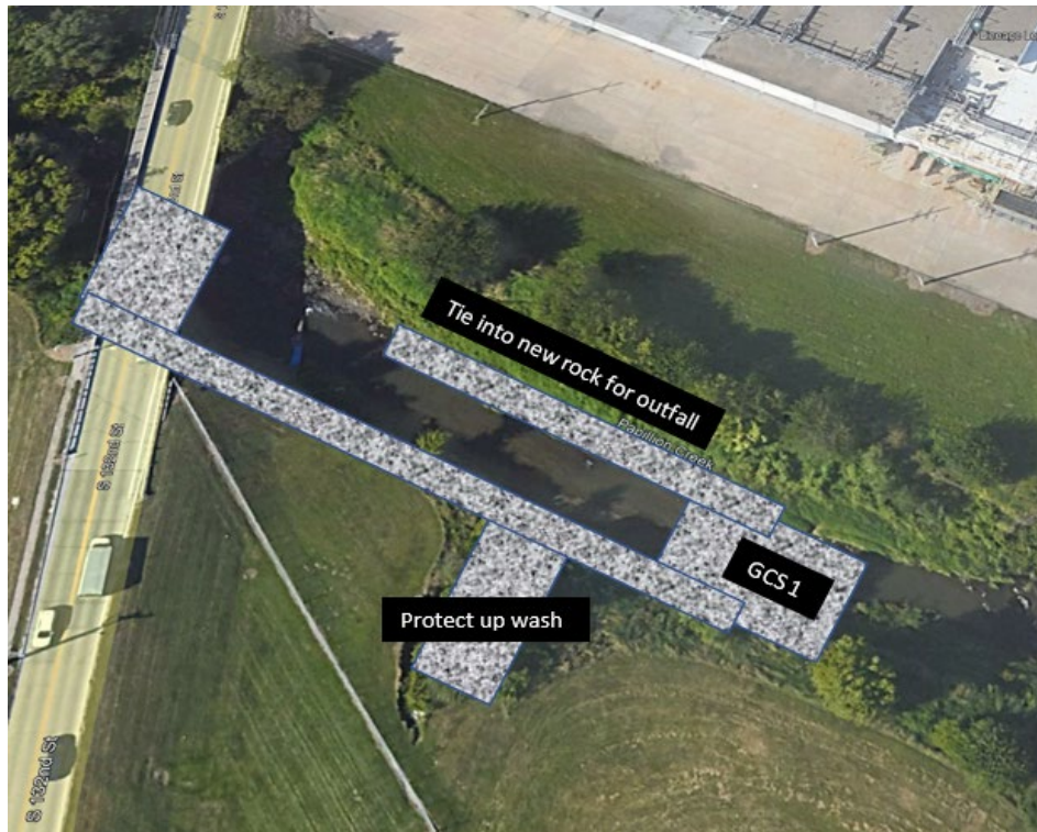
Figure 7-11: Conceptual Design of West Papillion Creek at 132 nd Street
